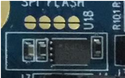
Figure 17: Optional external serial SPI flash IC (U18) schematic and PCB
