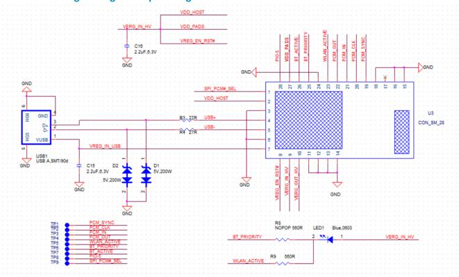
Figure 19: USB dongle design schematic
