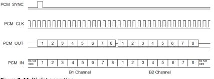
Figure 7: Multi-slot operation
