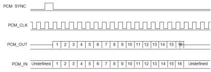
Figure 5: Short Frame Sync (Shown with 16-bit Sample)
