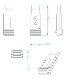
Figure 20: BT820 USB dongle, containing embedded BT800
