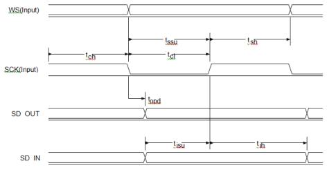
Figure 14: Digital audio interface slave timing
