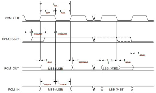
Figure 11: PCM Slave timing long frame sync
