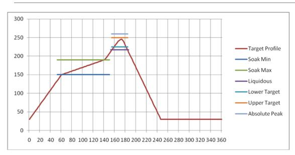
**Important**: During reflow, modules should not be above 260° and not for more than 30 seconds.
