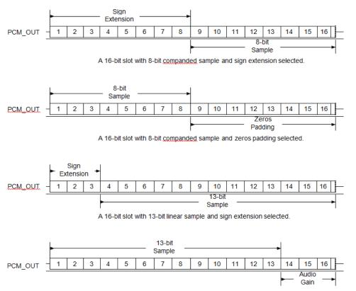
Figure 8: 16-bit slot length and sample formats
