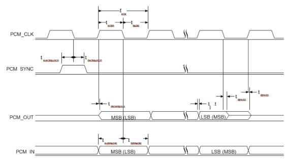
Figure 12: PCM Slave timing short frame sync
