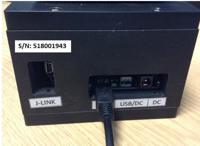
Figure 4: Connecting programming jig to a PC USB port
