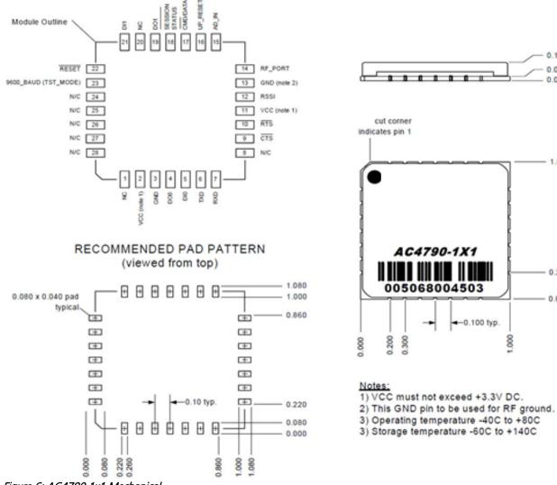
Figure 6: AC4790 1x1 Mechanical
