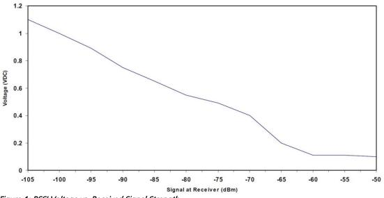
Figure 1: RSSI Voltage vs. Received Signal Strength
