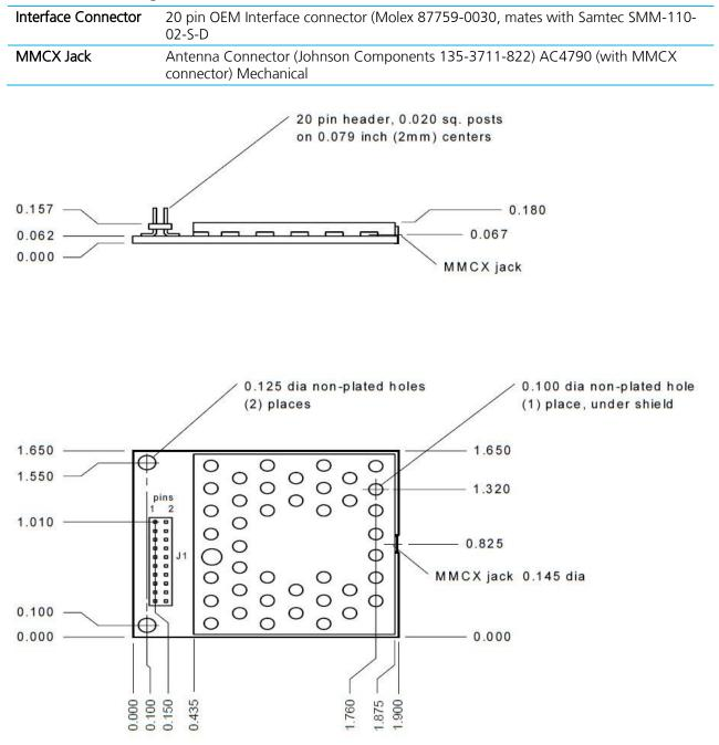
Figure 4: AC4790 (with MMCX connector) Mechanical
