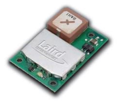
The Bluetooth® Intelligent Serial Module is specifically designed for applications where robust short range connectivity is required. This particular module provides a reliable Bluetooth connection that exceeds all requirements in terms of performance. The excellent range of up to 300 meters with very low power consumption of less than 36 mA makes this module a true class leader.
