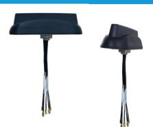
The Gar VFP69383B22JN multiport/multiband antenna provides an excellent solution for Public Safety, Transportation and Aftermarket Fleet applications. Configured for 2-port MIMO operation over the 3G/4G/ISM/CBRS bands and 2-port MIMO operation over the low//high frequency Wi-Fi bands. An additional 5<sup>th</sup> port provides an active antenna for enabling GNSS global navigation services.
