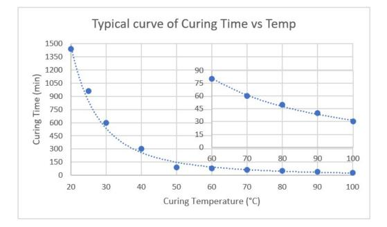
The above cure profiles are guideline recommendations. Cure conditions (time and temperature) may vary based on customers' experience and their application requirements, as well as customer curing equipment, oven loading and actual oven temperatures.
