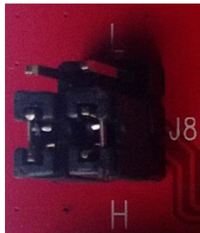
Figure 10: Configure the baud rate jumper
