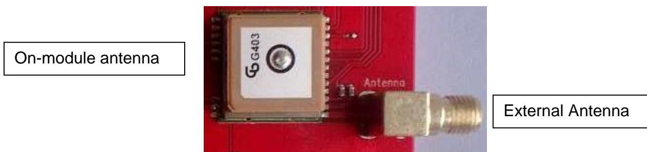
Figure 6: On-module antenna and External Antenna Connector
