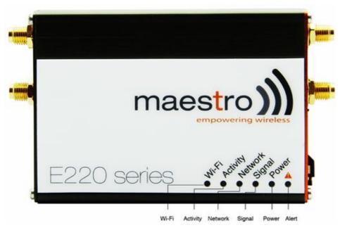
4.3.1 The top panel of Maestro's E220 Series features 6 LEDs on the front to indicate critical system information.
