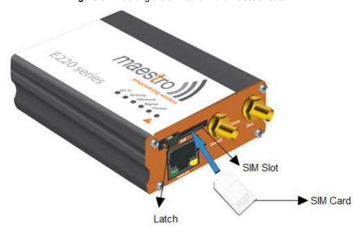
5.1.2 Connect the antenna to the main connector of the E220.
