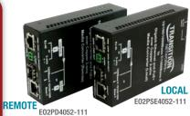
networks with modern PoE powered IP devices without the need to replace the existing copper wire infrastructure. The extenders leverage existing 18-24 AWG unshielded twisted pair (CAT 5, CAT 3 and other twisted 2-wire phone wire) cabling infrastructure to extend the Ethernet network at half Gigabit speeds and provide data and power to IP devices in remote locations, saving time and money over installing new cable.
