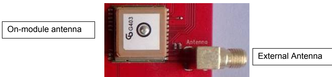
Figure 6: On-module antenna and External Antenna Connector
