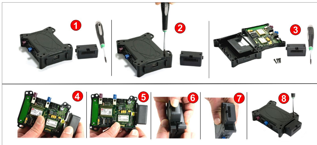
Figure 22: Mounting IOBOX-MINI or IOBOX-CAN/WLAN to the FOX3-2G/3G/4G devices.
