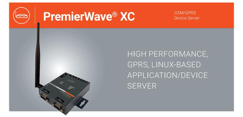
A high performance, multi-port secure device server that offers Ethernet or GSM/GPRS connectivity for remote access and easy management of machines and equipment over the network and across the Internet.
