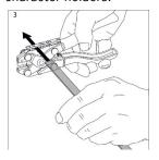
5. Use the front cutting part to cut the punched holders
