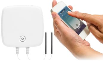
The EL-MOTE-DTP+ kit has been designed to monitor temperature in a large range of applications, using High Accuracy 75mm length barrel temperature probes on 3m cables. Ideal for monitoring locations perhaps difficult or inhospitable to the data logger itself, the EL-MOTE-DTP+ is ideal for monitoring refrigeration or storage units. This kit has 2 channels so you can monitor 2 separate areas simultaneously.
