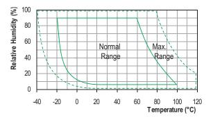
Long term exposure to humidity levels outside of the 'normal' range may temporarily offset RH measurements (±3%RH after 60 hours). Once returned to less extreme conditions the device will slowly return towards calibration state.
