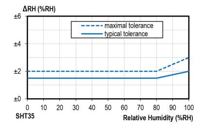
Typical tolerance of RH over Temperature:
