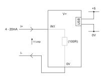
MEASURING 4-20mA USING A USB POWER SUPPLY
