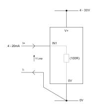
MEASURING 4-20mA Power supply to meter must be fully floating (isolated from the 4-20mA current loop)
