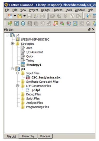
After this step, click **Process** at the bottom of window, then double-click **Place & Route Design** to Start PAR. This is similar to a standard Diamond PAR flow.
