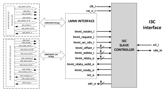
Figure 2.1. I3C Slave IP Core Functional Diagram
