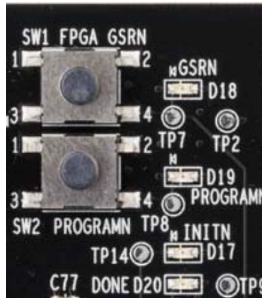
Figure 6. ECP5-5G Status LEDs and Push-button Controls
