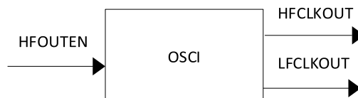
Figure 3.14. CrossLinkPlus OSCI Component Symbol
