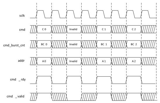
Figure 2.4. Timing of Command and Address
