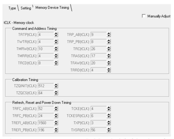
Figure 3.3. DDR2 SDRAM IP Core Memory Device Timing Options in the Clarity Designer Tool
