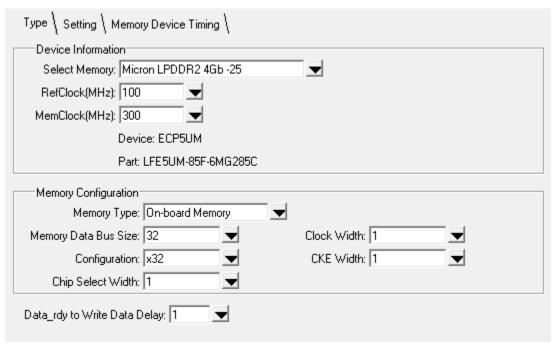
Figure 3.1. LPDDR2 SDRAM Controller Lite IP Core Type Options in the Clarity Designer Tool
