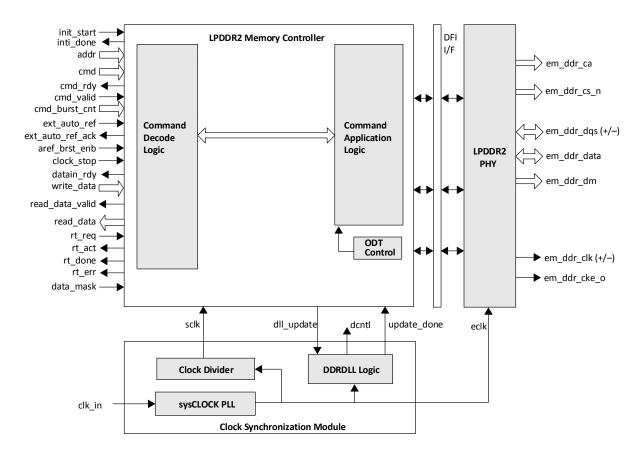
Figure 2.1. LPDDR2 SDRAM Controller Lite Block Diagram
