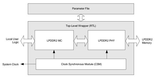
Figure 4.5. File Structure of LPDDR2 Memory Controller IP
