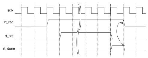
Figure 2.3. Timing Diagram for Read Retraining
