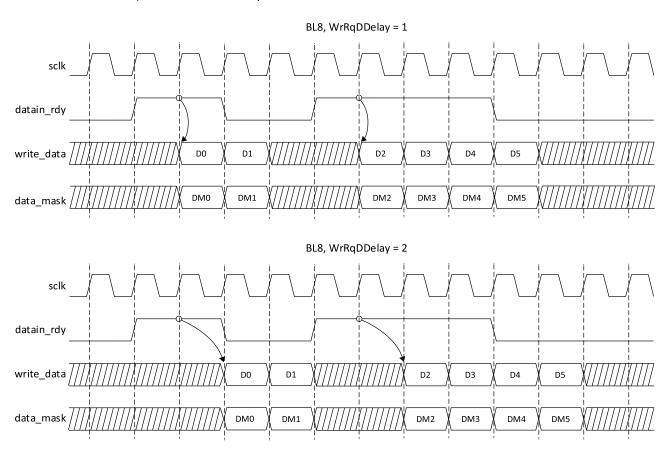
Figure 2.5. Timing One-Clock vs. Two-Clock Write Data Delay
