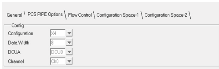
Figure 3.2. PCI Express IP Core PCS Pipe Options
