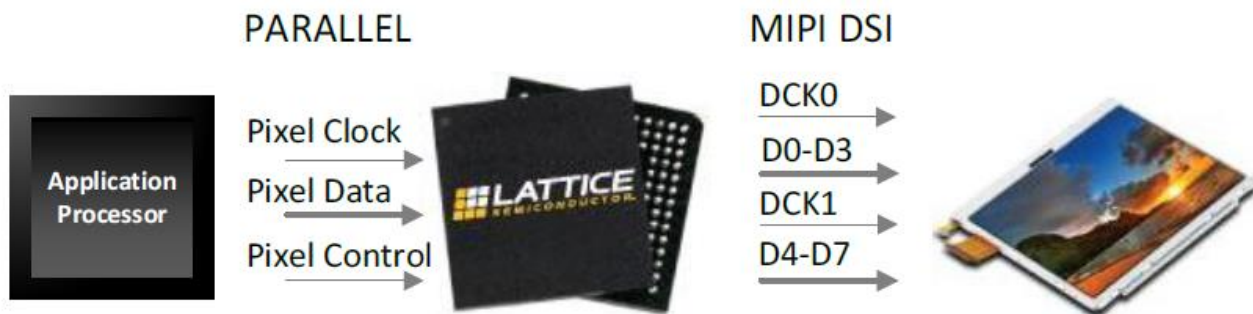
Figure 1.1. Sample Parallel Interface to MIPI DSI System Diagram
