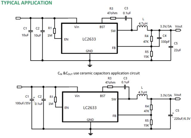
$C_{\text{IN}}$  &C\_{\text{OUT}} use electrolytic capacitors application circuit
