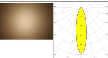
CLU700/701/702 LED  $\mathsf{FWHM}\,/\,\mathsf{FWTM}$ 20.0° / 58.0° Efficiency 79 % Peak intensity 3.1 cd/lm LEDs/each optic Light colour White Required components:
