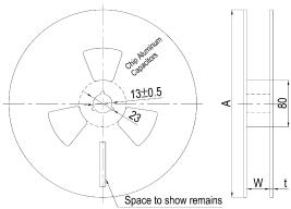
Fig. 2-2 Reel Polarity
