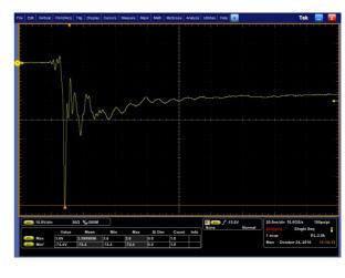
Fig 4 .Negative 8kV contact per IEC61000-4-2
