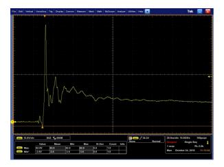
Fig 3 .Positive 8kV contact per IEC61000-4-2
