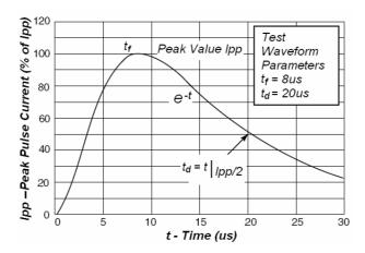
Fig3. Pulse Waveform
