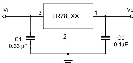
Note 1: To specify an output voltage, substitute voltage value for "XX".
