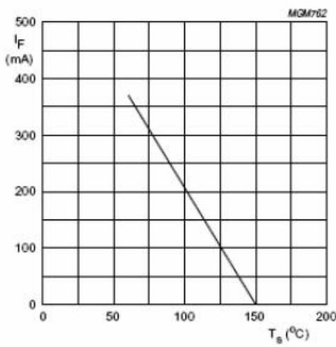
Fig.2 Maximum permissible continuous forward current as a function of soldering point temperature.
