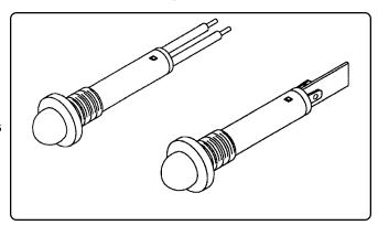
Black Housing Dome Lens Variety of Lens Colors Hex Nut Threaded Housing
