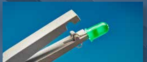
RX 601 forming pliers leave a standoff in wire and on LED leads.
