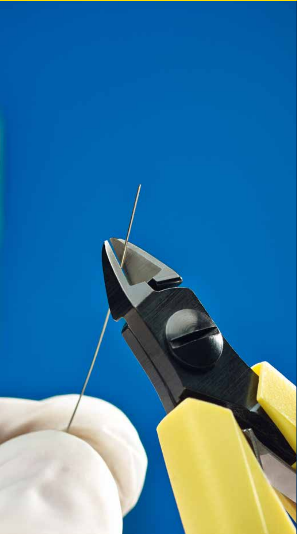
8154PSP cutter used to trim a stent.
