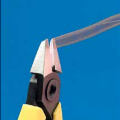
8154PSP cutter used to trim a stent.
