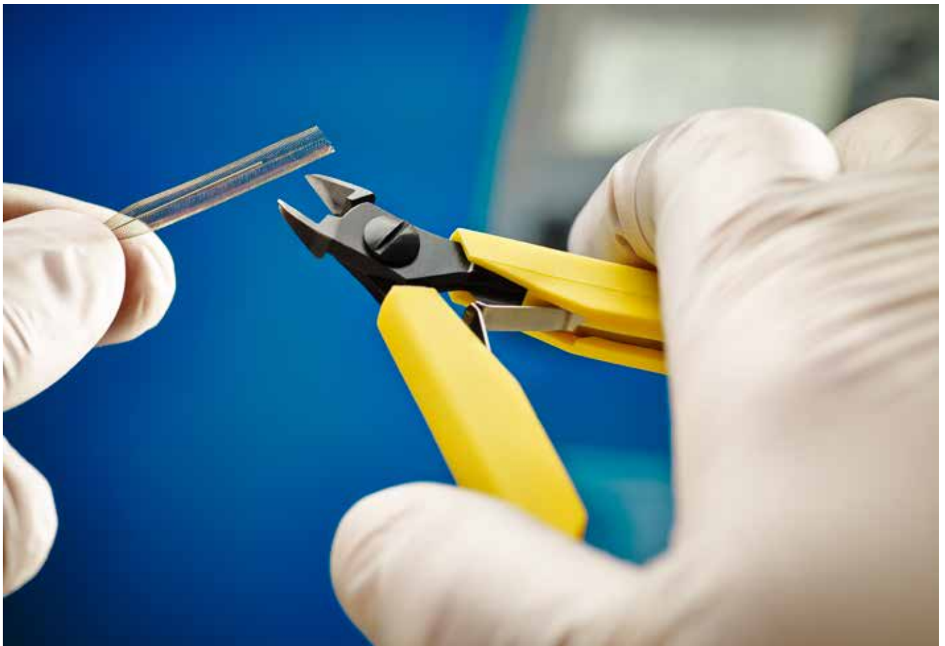
Stents can be trimmed with Lindström 8130 cutters.
