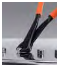
Nut pliers are intended to use for gripping small nuts (counter grip) in confined spaces.
