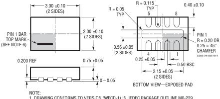
DDB Package 8-Lead Plastic DFN (3mm × 2mm) (Reference LTC DWG # 05-08-1702 Rev B)
