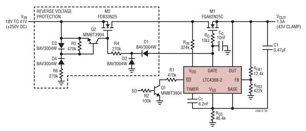
Figure 8. 28V Vehicle Application with Reverse Voltage Protection
