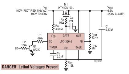
Figure 7. Rectified 110V AC Supply Protected from 220V AC
