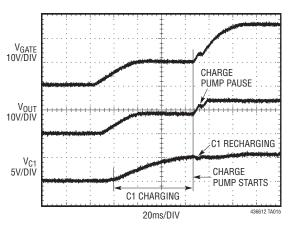
Figure 2. Turn-On Waveforms
