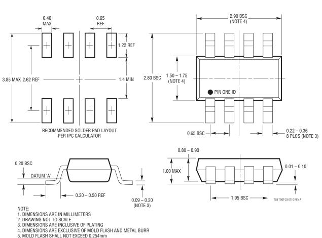
TS8 Package 8-Lead Plastic TS0T-23 (Reference LTC DWG # 05-08-1637 Rev A)
