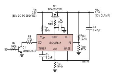
Figure 6. Overvoltage Protected 28V, 1.5A Supply
