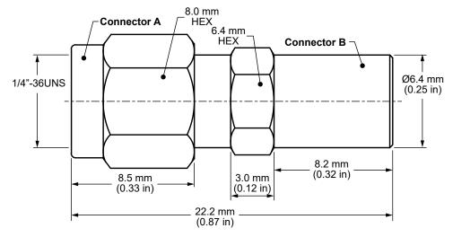
Figure 1. Product Dimensions for the ADP-SMAM-SMBM-G Adapter
