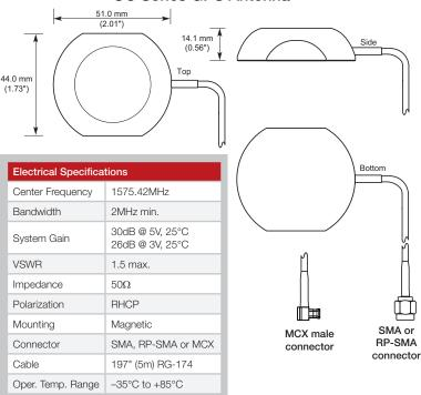
xxx = Insert "SMA", "RPS" or "MCX" for SMA, RP-SMA or MCX connector
