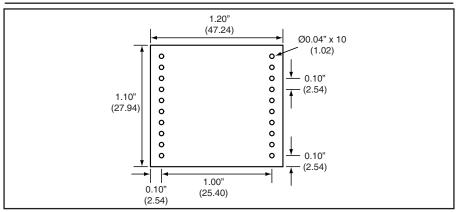
Figure 2: MDEV-GPS-SG-DB PCB Layout Dimensions
