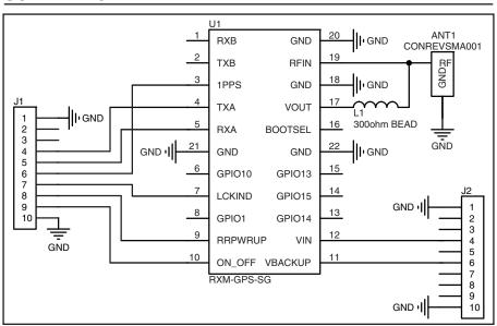
Figure 3: MDEV-GPS-SG-DB Schematic
