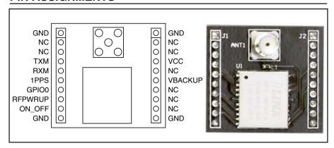
Figure 1: MDEV-GPS-SG-DB Pin Assignments
