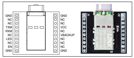
Figure 1: MDEV-GPS-SR-DB Pin Assignments
