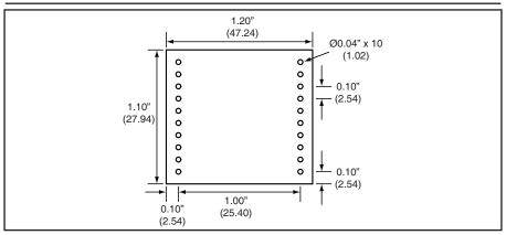
Figure 2: MDEV-GPS-SR-DB PCB Layout Dimensions
