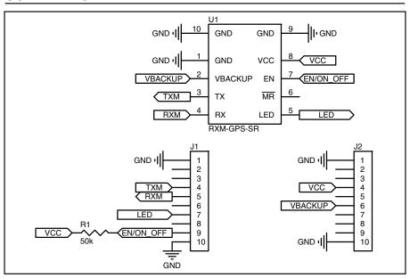
Figure 3: MDEV-GPS-SR-DB Schematic
