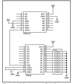
Figure 6: LR Receiver and HT658 Schematic
