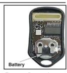
Figure 4: Battery Access
