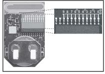
If the trace is intact, the address line is connected to ground, otherwise it is
