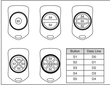
Figure 3: CMD-KEY#-\*\*\* Button Assignments
