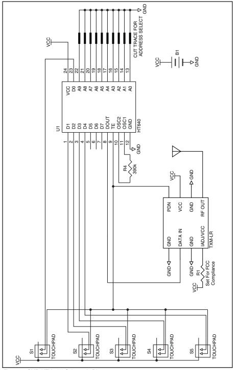
Figure 7: CMD-KEY#-\*\*\* Schematic Diagram
