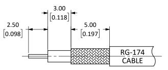
RECOMMENDED CABLE STRIPPING DIMENSIONS CAN ALSO BE USED WITH: RG-188A & RG-316
