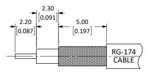
RECOMMENDED CABLE STRIPPING DIMENSIONS CAN ALSO BE USED WITH: RG-188A & RG-316
