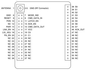
Figure 5: EVM-xxx-RC Pin Assignments
