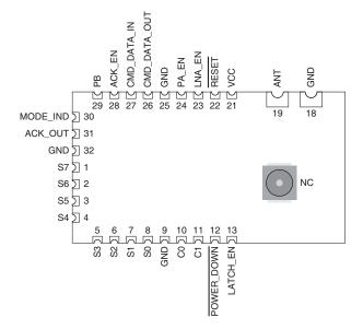
Figure 14: HumPRCTM Series Transceiver Pre-certified Version Pin Assignments - Castellation Connection (Top View)
