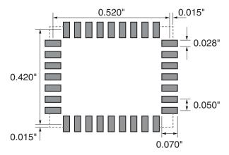
Figure 95: HUM-\*\*\*-PRC Recommended PCB Layout
