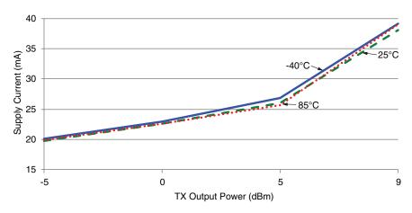
Figure 6: HumPRC™ Series Transceiver Average Current vs. Transmitter Output Power at 2.5V
