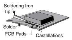
Figure 100: Soldering Technique
