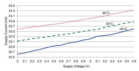
Figure 10: HumPRC™ Series Transceiver RX Scan Current vs. Supply Voltage, 9.6kbps
