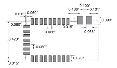
Figure 96: HUM-\*\*\*-PRC-UFL/CAS Recommended PCB Layout
