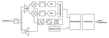
Figure 20: HumPRC™ Series Transceiver RF Section Block Diagram
