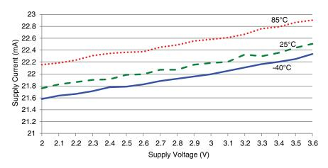
Figure 11: HumPRC™ Series Transceiver RX Scan Current vs. Supply Voltage, 115.2kbps
