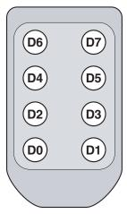
Figure 6: OTX-\*\*\*-HH-CP8-MS Button Assignments
