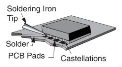
Figure 29: Soldering Technique
