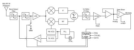
Figure 19: LT Series Transceiver Block Diagram
