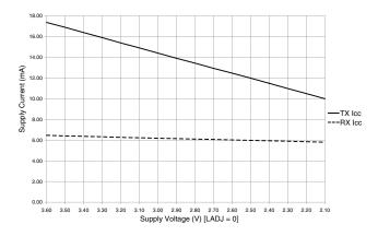
Figure 8: Current Consumption vs. Supply
