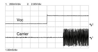
Figure 15: TX Turn-On Time from  $V_{\rm cc}$
