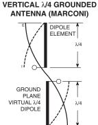
Figure 33: Dipole Antenna
