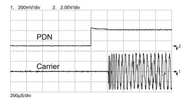
Figure 14: TX Turn-On Time from PDN
