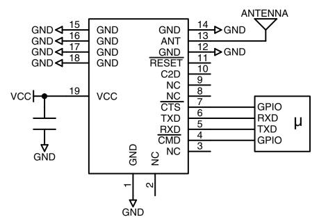
The DTS and EUR Series Transceivers are configured through a UART interface.
