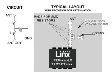
Figure 14: A T-Pad Attenuator Layout Example
