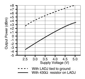
Figure 6: Output Power vs. Supply Voltage
