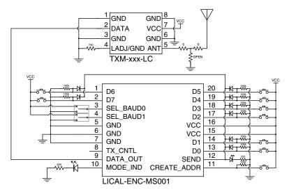
Figure 16: LC Series Transmitter and MS Series Encoder
