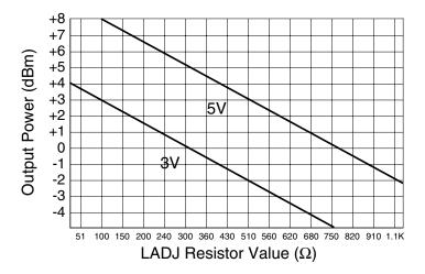
Figure 9: Output Power vs. LADJ Resistor
