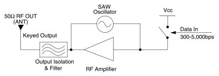
Figure 12: LC Series Transmitter Block Diagram
